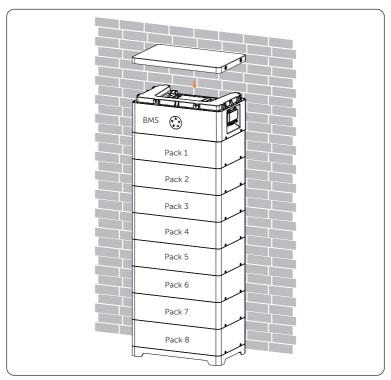
Figure 6-34 Placing BMS
