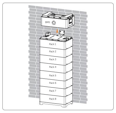
Figure 6-14 Placing BMS
