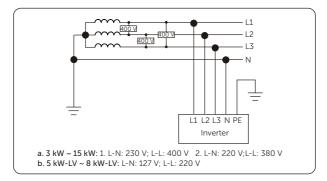
Figure 2-2 Supported power grid - TT
