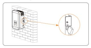
Figure 7-12 Locking the inverter
