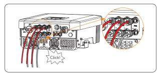
Figure 8-23 Connecting the PV cables
