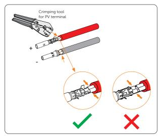
Figure 8-17 Crimping the PV cables with pin contacts
