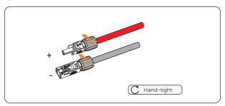
Figure 8-20 Tightening swivel nuts of PV connectors
