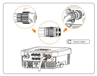
Figure 8-13 Connecting with the inverter
