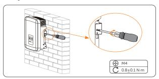
Figure 7-11 Securing the inverter
