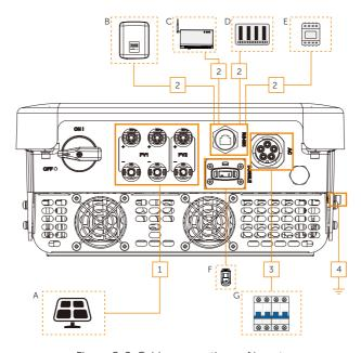
Figure 8-2 Cable connections of inverter
