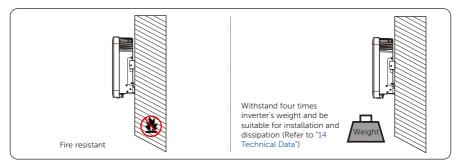
Figure 5-3 Installation carrier requirement
