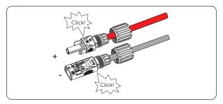
Figure 8-19 Securing the PV cables
