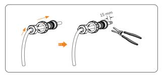
Figure 8-30 Threading and stripping the communication cable
