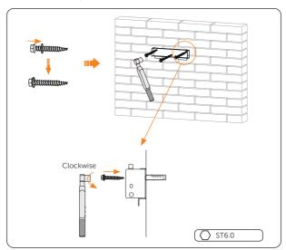
Figure 7-9 Securing the bracket
