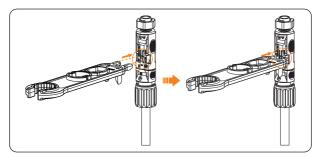
Figure 8-26 Disassembling the PV connectors
