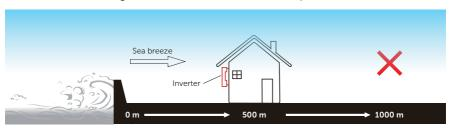
Figure 5-2 Incorrect installation position
