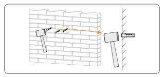
Figure 7-8 Inserting the expansion tubes
