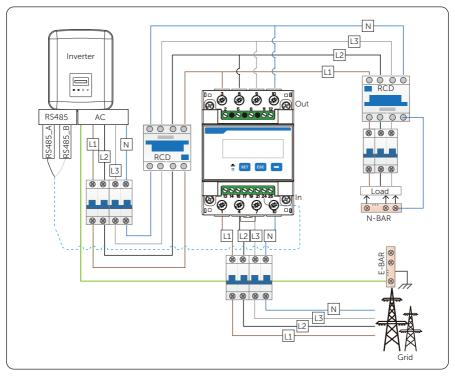
Figure 8-36 Meter connection diagram
