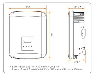
Figure 7-3 Dimensions 1 (Unit: mm)
