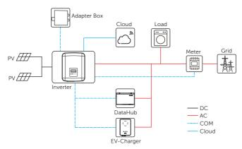
Figure 3-1 System diagram
