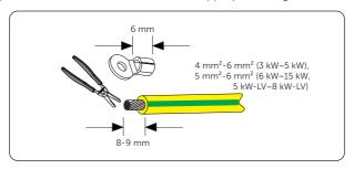
Figure 8-3 Stripping the PE cable
