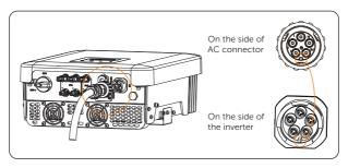
Figure 8-12 Aligning with the inverter
