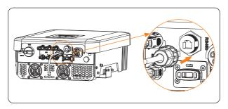
Figure 8-34 Connecting to the inverter
