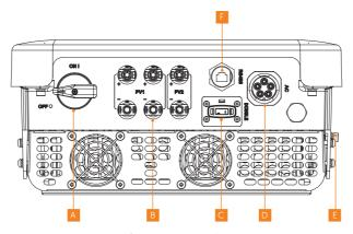
Figure 8-1 Terminals of Inverter
