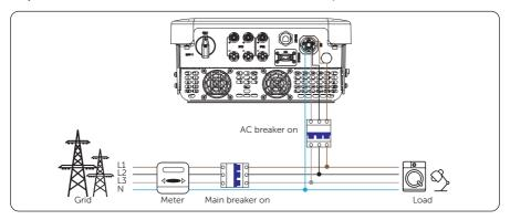
Figure 9-2 Switch on AC breaker
