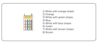
Figure 8-28 Pin of RS485 terminal
