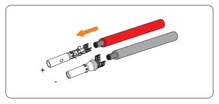
Figure 8-16 Inserting into the PV pin contact
