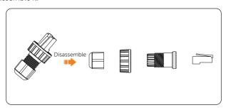
Figure 8-29 Disassembling the waterproof connector with RJ45
