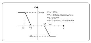
Figure 10-5 Curve Q = f(V)
