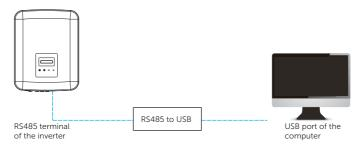
Figure 8-27 Communicating with computer
