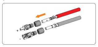
Figure 8-18 Threading the PV cables
