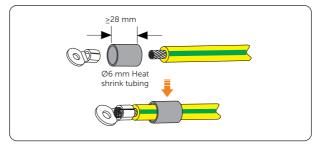
Figure 8-4 Installing the tubing and terminal
