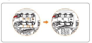
Figure 8-25 Disassembling the dustproof buckles
