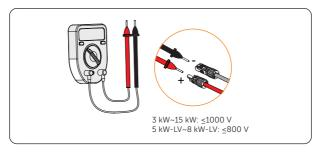
Figure 8-21 Measuring the voltage of PV connectors
