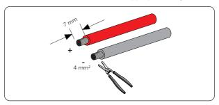
Figure 8-15 Stripping the PV cables
