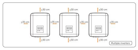
Figure 5-5 Clearance requirement for multiple inverters
