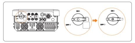
Figure 9-7 Unlocking the lockable DC switch
