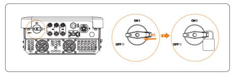
Figure 9-6 Locking the lockable DC switch
