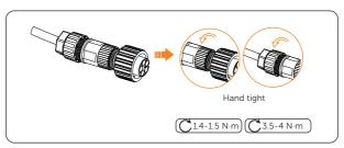
Figure 8-11 Tightening the connector
