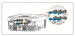
Figure 8-22 Removing the caps
