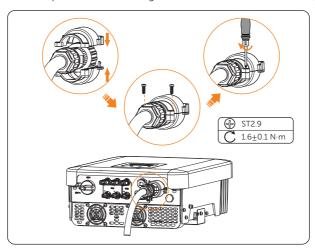
Figure 8-14 Installing the AC terminal sheath
