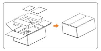
Figure 13-3 Packing the inverter
