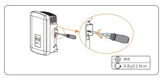
Figure 7-5 Unscrewing the bracket
