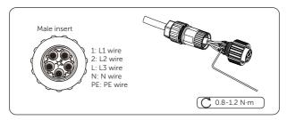
Figure 8-10 Securing the wires
