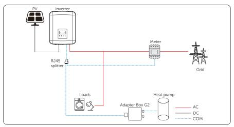
Figure 15-5 Adapter Box G2 wiring diagram
