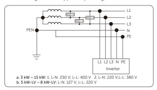
Figure 2-4 Supported power grid - TN-C-S
