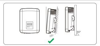
Figure 7-1 Correct installation
