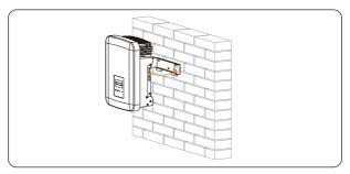
Figure 7-10 Lifting up and hanging the inverter
