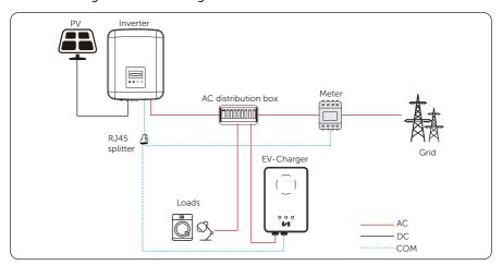
Figure 15-3 EV-Charger wiring diagram
