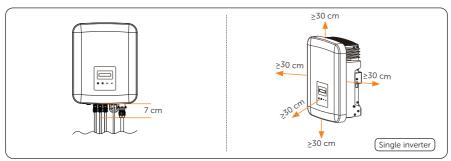
Figure 5-4 Clearance requirement for single inverter
