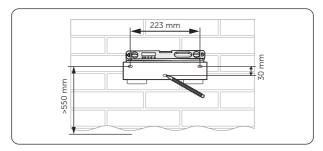
Figure 7-6 Marking the holes
