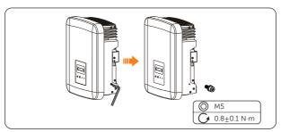
Figure 8-6 Removing the screw
