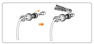
Figure 8-31 Crimping the RJ45 connector
