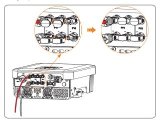
Figure 8-24 Sealing the unused PV terminals
