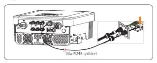
Figure 15-4 Connecting to EV-Charger
