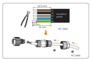
Figure 8-9 Stripping and threading the AC cable
