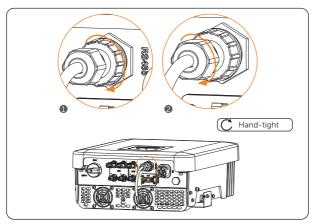
Figure 8-35 Tightening the waterproof connector
