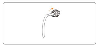
Figure 8-32 Reassembling the waterproof connector but not tightening
