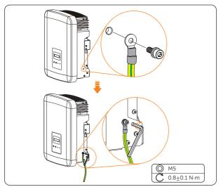
Figure 8-7 Securing the PE cable
