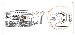
Figure 8-33 Removing the protective cover
