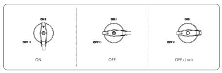
Figure 9-3 States of the lockable DC switch
