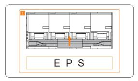
Figure 2-19 Flipping up EPS breaker
