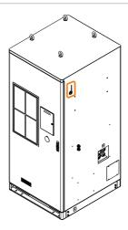
Figure 4-1 Position of the antenna
