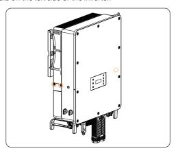
Figure 28-1 Dismantling screws
