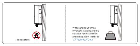
Figure 4-6 Installation carrier requirement
